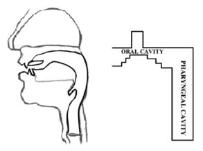
Figure 2. The articulatory scheme of the resonator for [1] and its approximation by a tube model (the side branch made by the tongue pocket is shown in both models)
